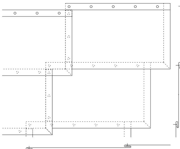
Detail of the façade-panel fixation. Scale 1:10.
